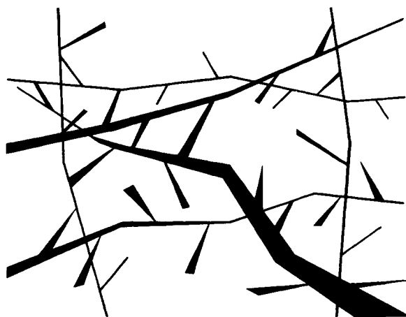
Figure 6. Schematic of the two-step rigid network gel in perspective. The network is constructed from stiff linear polyamide chains and an excess of rigid connector species. Solvent is not shown. Additional explanations are given in the text.
